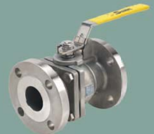
150#, 300#, 600# Flanged Ball Valves Full & Reduced Port Carbon Steel, 316 Stainless & Alloy 20 1/2" - 12"
